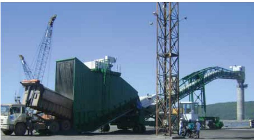
Figure 2: a single, inline SAMSON material feeder with integrated shiploader
