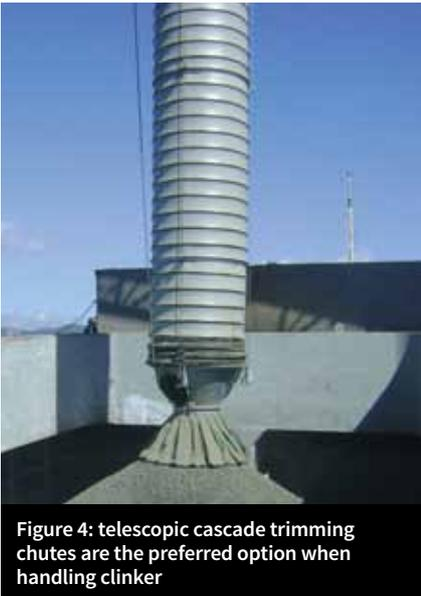
Figure 4: telescopic cascade trimming chutes are the preferred option when handling clinker
