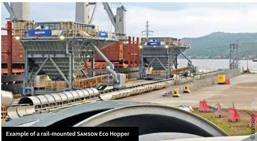
Example of a rail-mounted SAMSON Eco Hopper
